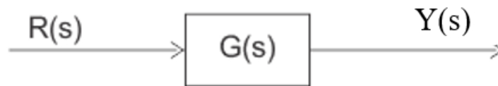
Figure 3.3: Representation of the relationship between the input and output of a system in the Laplace domain.
