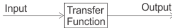
Figure 3.2: The relationship between the input and the output of a system is defined as transfer function.
