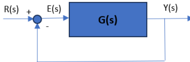
Figure 5.1: Block diagram representation of the Unity feedback system.
